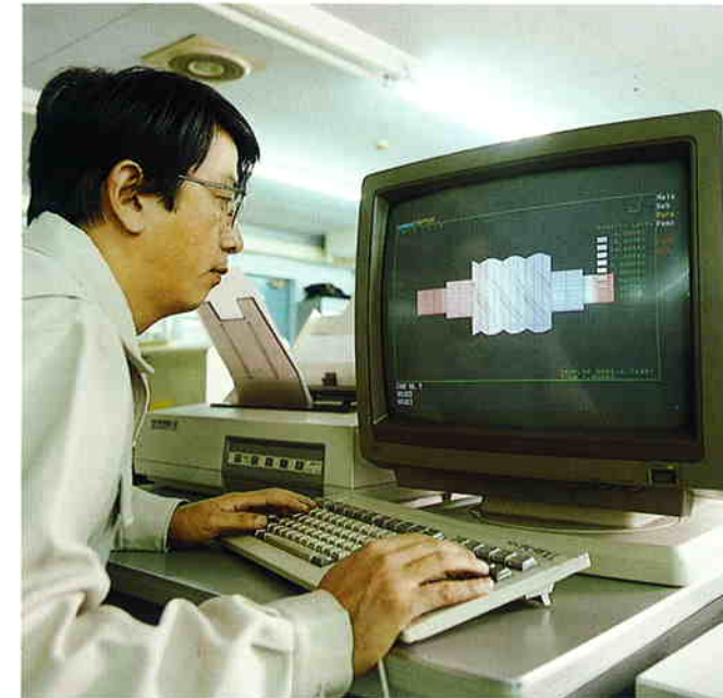
Rotor Thermal Distortion Analysis, Monitored with Finite Element Method
